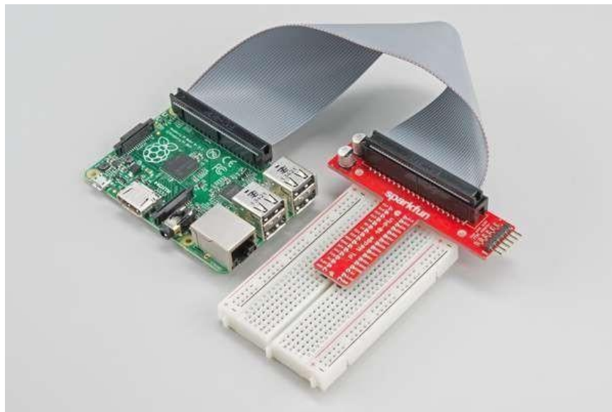
The Pi Wedge helps access the I2C and SPI signals.
